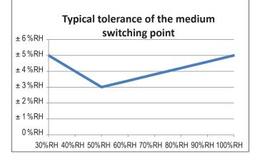
1-point-adjustment at 48 % RH/23 °C Long-term drift: ≤±1 % RH p.a.
